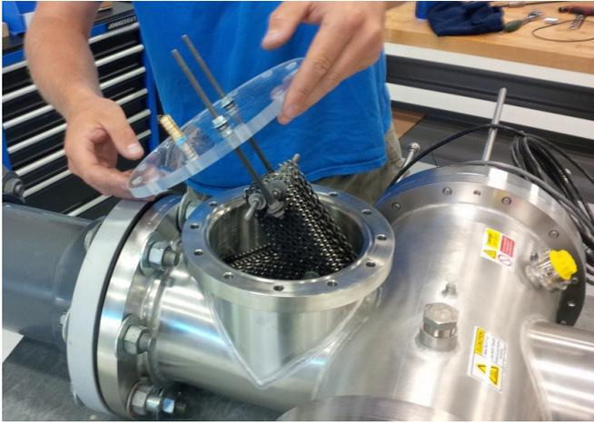
Figure 3. Electrode assembly being inserted into an ETS-UV™ AOP system, directly upstream of the UV lamps
