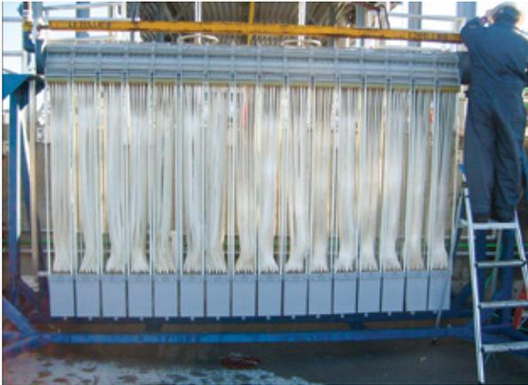
MEMCOR® B40N hollow fiber membranes deliver greater filtration performance and reduce energy up to 60 percent
