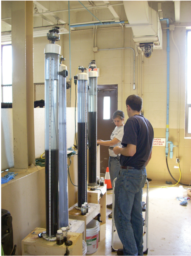
Bench tests can be performed on site to quantify the settling enhancement of the process.
