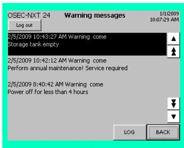
The "i" (Info) button allows you to view the current warning messages that have been displayed by the system, including the date, time and status details ("come"), at any time.
