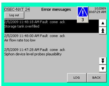
The "i" (Info) button allows you to view the error messages that have been displayed by the system, including the date, time and status details ("come", "ack" and "gone"), at any time.
