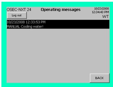
Which of these manual functions is currently active can be displayed in the operating messages menu by pressing the "i" (Info) button.
