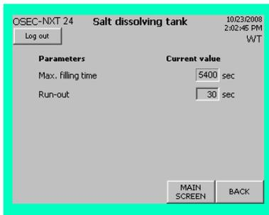
The "Salt dissolving tank" menu is used to enter limits for the max. filling time and run-out time for the salt dissolving tank. If the values entered here are exceeded an error message is generated.
