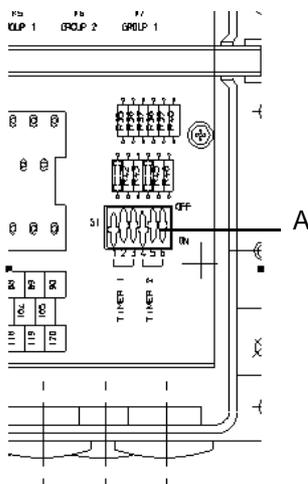
1 The DIP switches (A) must be set as follows (to the right of the terminals box):
