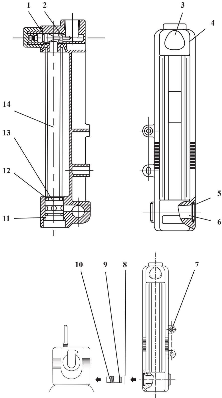
FIG.2B FLOWMETER ASSEMBLY 125mm
