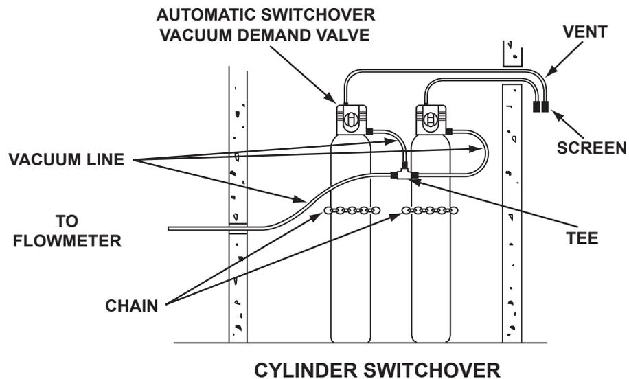
When mounted on a gas supply cylinder, the vacuum demand valve is connected to the cylinder valve by a yoke. The cylinder must be in the upright position with the cylinder valve on top as shown on the sketch shown above.
