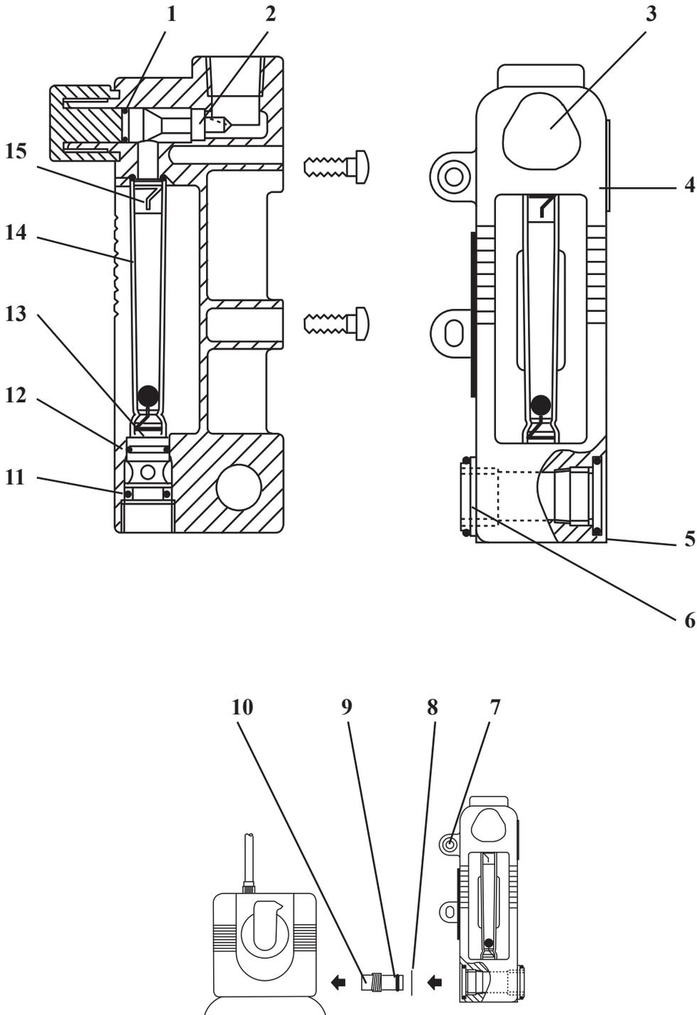
FIG.2A FLOWMETER ASSEMBLY (75mm)
