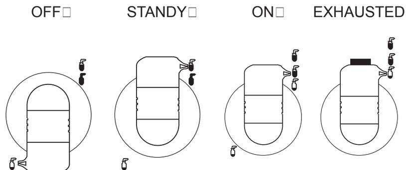
**ON:** (valve open): indicated by a shaded-in cylinder outline without the bar and showing gas flowing through the supply pipeline.
