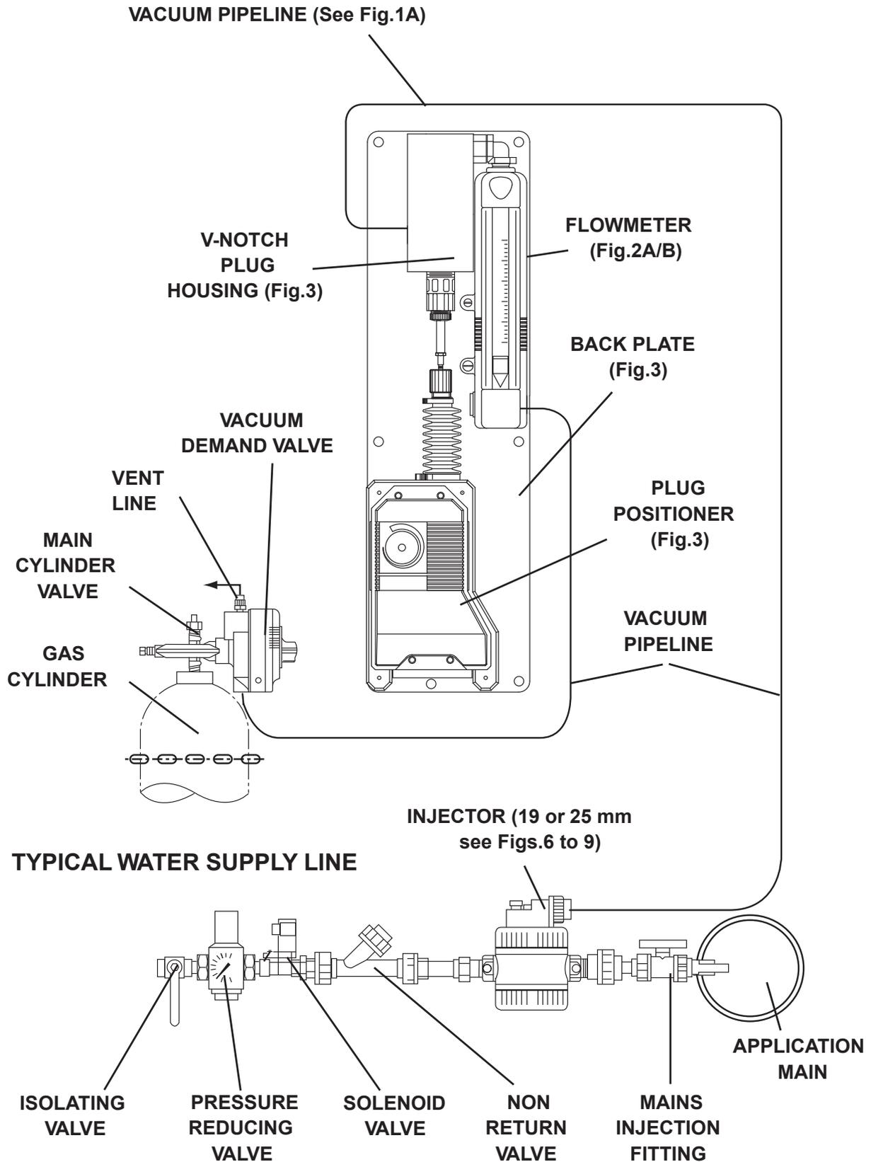
**FIG.1B TYPICAL LAYOUT (AUTOMATIC CONTROL UNIT)**
