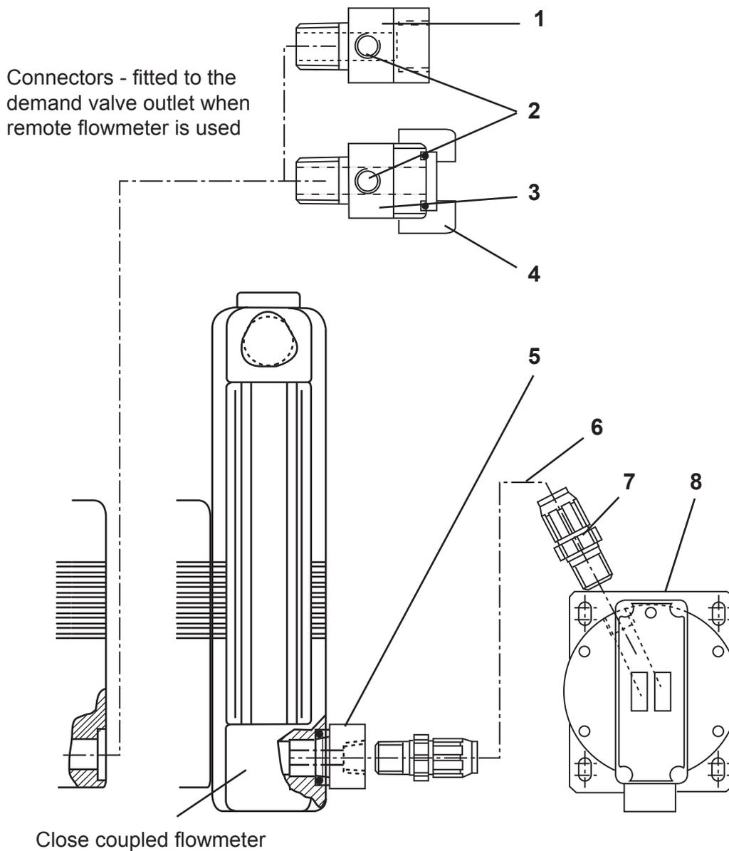
**FIG.11 REMOTE MOUNTED ALARM SWITCH**
