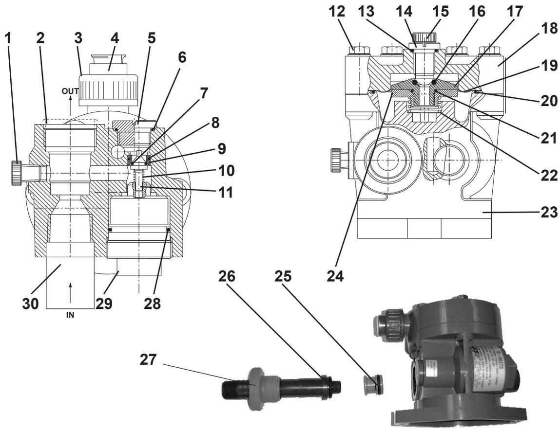
FIG.6 U.96273 - STANDARD 25mm INJECTOR
