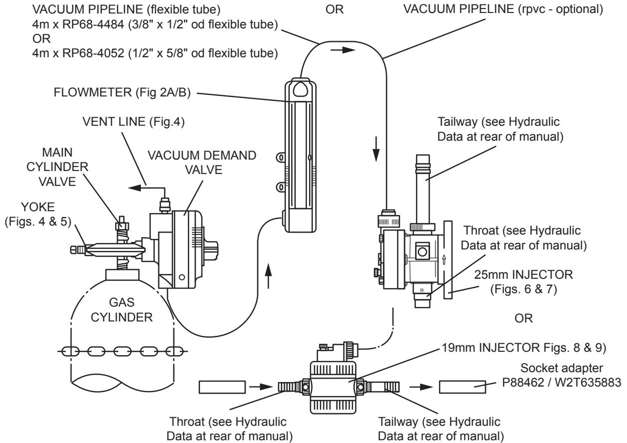
**FIG.1A TYPICAL LAYOUT (REMOTE MOUNTED FLOWMETER)**
