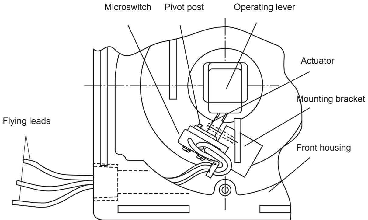
**FIG.10 INTERNAL ALARM SWITCH**
