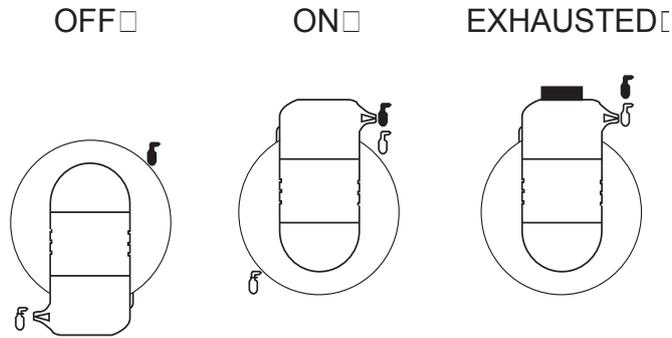
**SUPPLY EXHAUSTED:** (valve open but cylinder empty): indicated by an empty cylinder outline with bar removed but no flow of gas in the supply pipeline. In this position the red OUT OF GAS warning indicator, located immediately above the top of the knob, is also uncovered.
