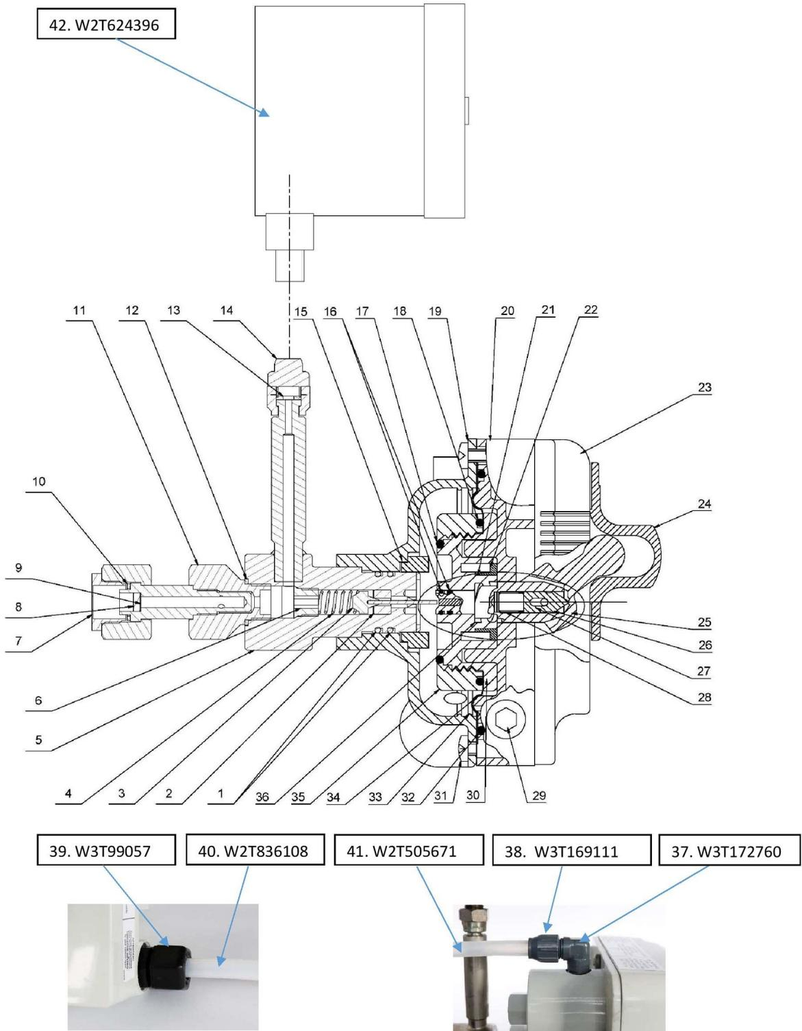
**FIG. 17 S10k DIRECT MOUNT CHLORINE VACUUM REGULATOR (No. 6 CONNECTION)**
