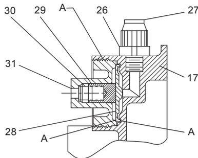
**FIG.16 VACUUM DEMAND VALVE (running nut)**
