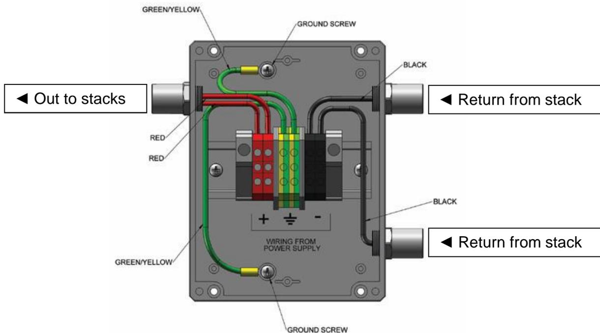
Figure 3-5 Inside the VNX Junction Box (2-stack module)
