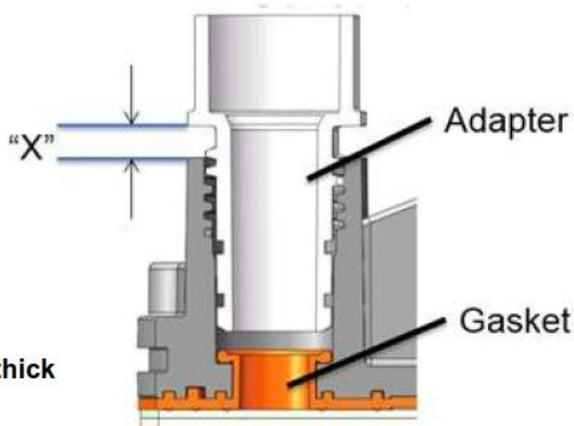
**Figure 3-4 Proper Tightening of VNX Piping Adapter**
