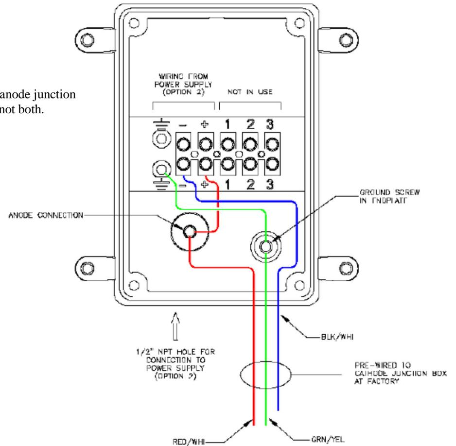
WIRING INSIDE ANODE JUNCTION BOX
