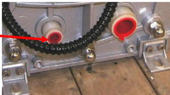
**Figure 3-1b LX-EU, LX-X, LX-Z modules (BSPM) with red shipping plugs**
