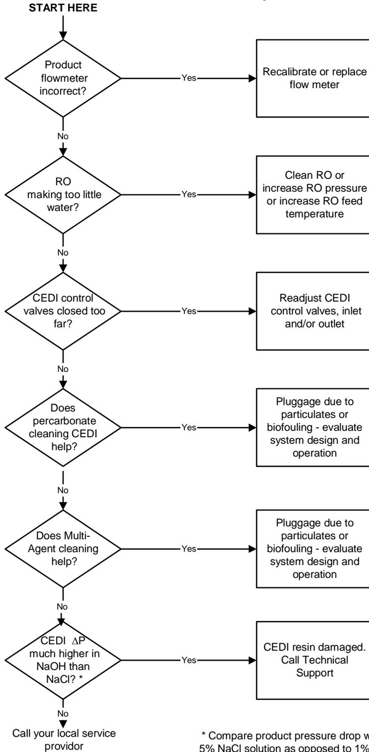
\* Compare product pressure drop when circulating 5% NaCl solution as opposed to 1% NaOH solution
