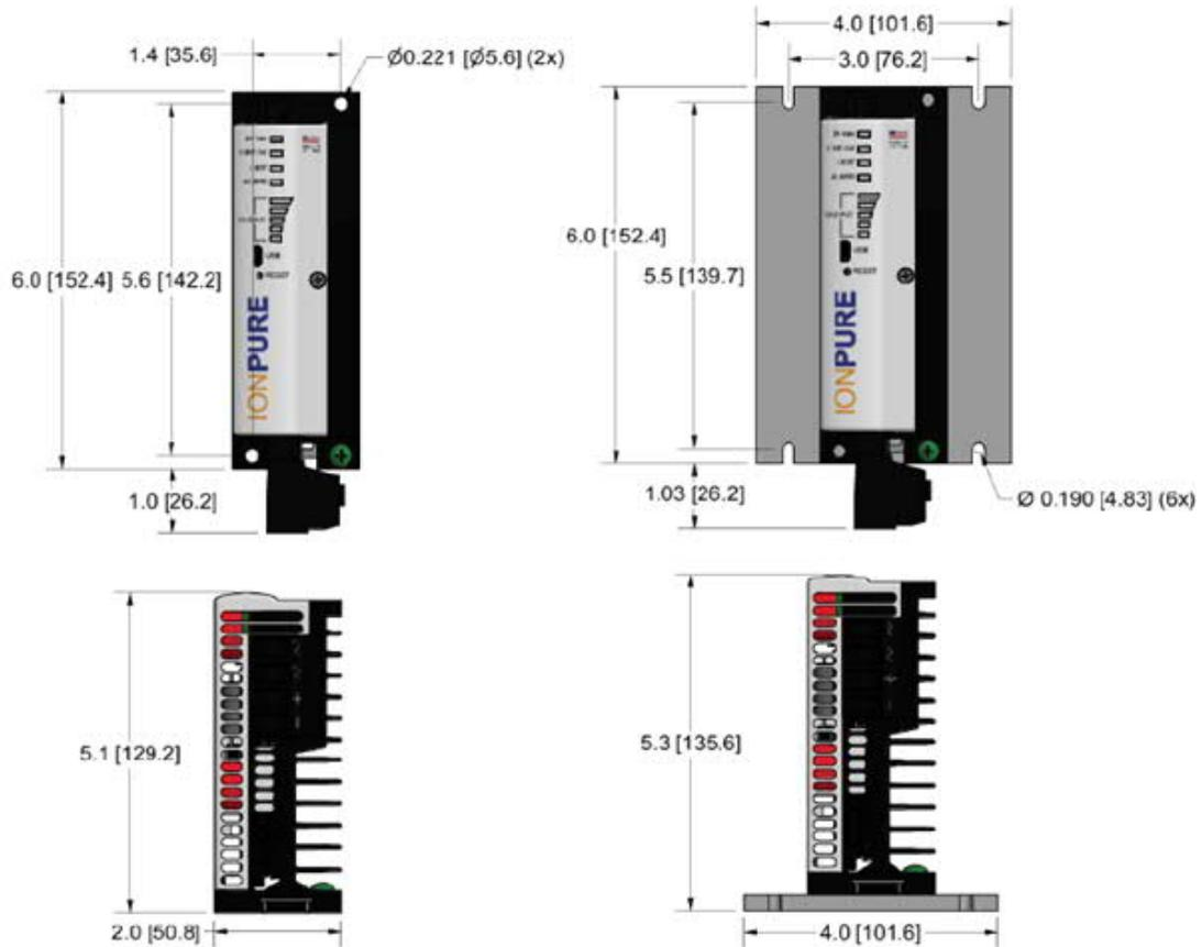
The environmental limits for operation are 0 to 50 °C, at up to 95% relative humidity (non-condensing). An enclosure with at least an IP52/NEMA 12 rating is recommended. The DCR contains a heatsink for cooling; however, the enclosure should also include a cooling fan that draws through ambient air.
