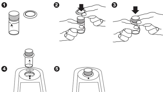
1. Always perform zeroing and test with closed vial cap. Only use cap with sealing ring.
