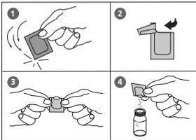
5. Add the contents of **one VARIO Chlorine FREE-DPD / F10 Powder Pack** straight from the foil to the water sample.
