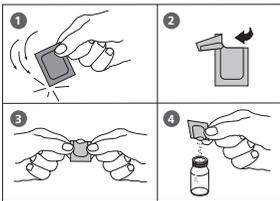
5. Add the contents of **two Vario Chlorine Free-DPD/ F10 Powder Pack** straight from the foil into the water sample.
