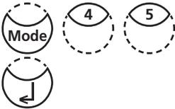
If the test result is displayed press [MODE], [Shift] + [4] [5] keys and confirm with [↵] key.
