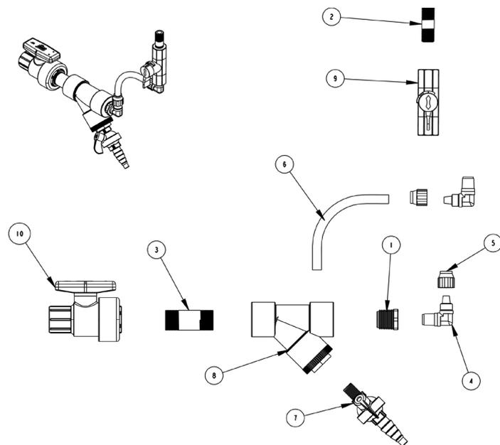
Figure 2.5 MICRO/2000® and DEOX/2000® sample line
