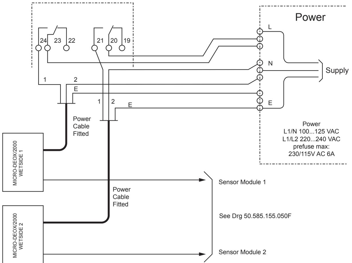
MFC - SCHEMATIC WIRING
