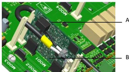
Fig. 12 Section ORP sensor module with sensor cable in slot
