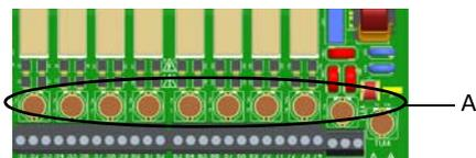
Fig. 3 Section, electronics module - fuses
