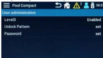
The parameter Level 1/Level 2 or Level 3 is used to enable or disable user level 1,2 and 3. Enter the setting "enabled" to use the Level. After enabling, an unlock pattern and/or password for login must be defined (at least one of these two login options must be set).
