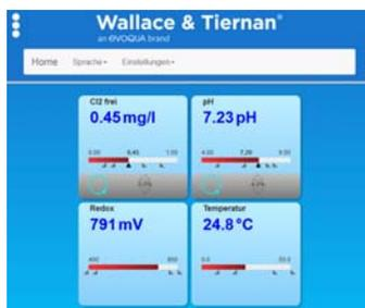
Fig. 3 Example, web view DEPOLOX® Pool Compact
