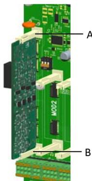
Fig. 11 View, installation of the 4-way mA output card
