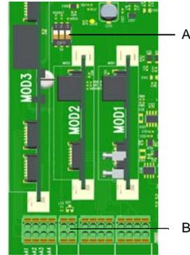
Fig. 2 Detail of PCB - RS485 interface
