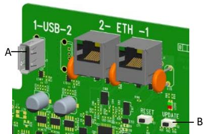
Fig. 4 Section, circuit board
