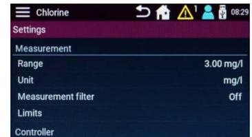
Depending on the measurement selected, different setting parameters are displayed. Swipe upward on the touchscreen to access further setting parameters which are further down the list and not currently visible on the screen.
