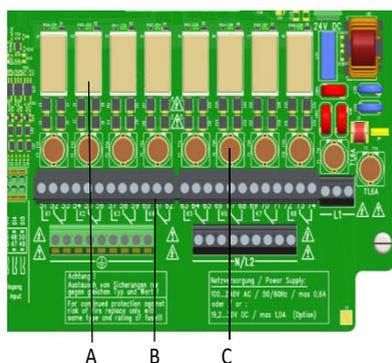
Fig. 5 Detail of PCB - relay outputs
