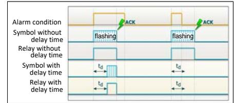
Fig. 3 Acknowledgment “ACK with reset”
