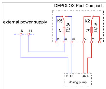
Fig. 10 Plan of terminal assignment
