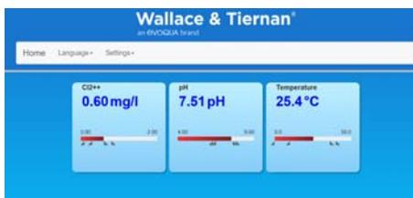
Fig. 3 Example, web view DEPOLOX® 400 M
