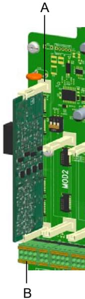
Image 10 View, installation of the 4-way mA output card
