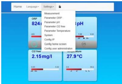
User administration via web visualization comprises two levels. At the factory, these two user levels are disabled and preset to “0”. For security reasons, the user levels must be enabled during commissioning. The padlock symbol in the menu bar shows whether the user is logged in. Depending on the specific user, the various menus are shown or hidden.
