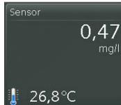
The menu field „Sensor” shows the current measuring value for chlorine with unit. The current sample water temperature is displayed underneath with a temperature symbol.
