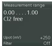
The menu field „Measurement range” shows the currently set measurement range for chlorine and the selected sensor type. The selected potential voltage Upot and the set measuring value filter are also shown.
